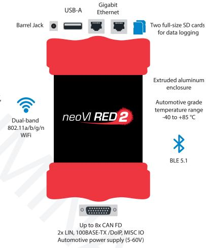
The neoVI RED 2 also has a real-time clock for hardware timestamping of all messages. A robust power management system automatically powers down the neoVI RED 2 and it wakes up again based on network activity or the connection of a PC.
